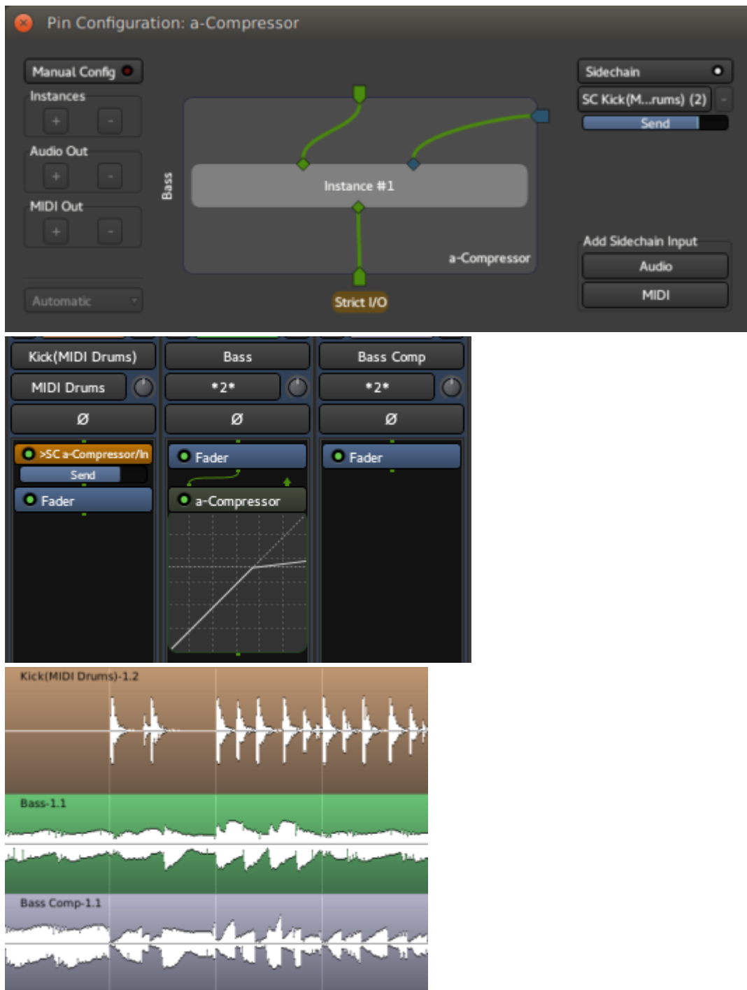
Fig. 69.19 - A sidechain compression: Pin configuration, mixer view and editor view.
