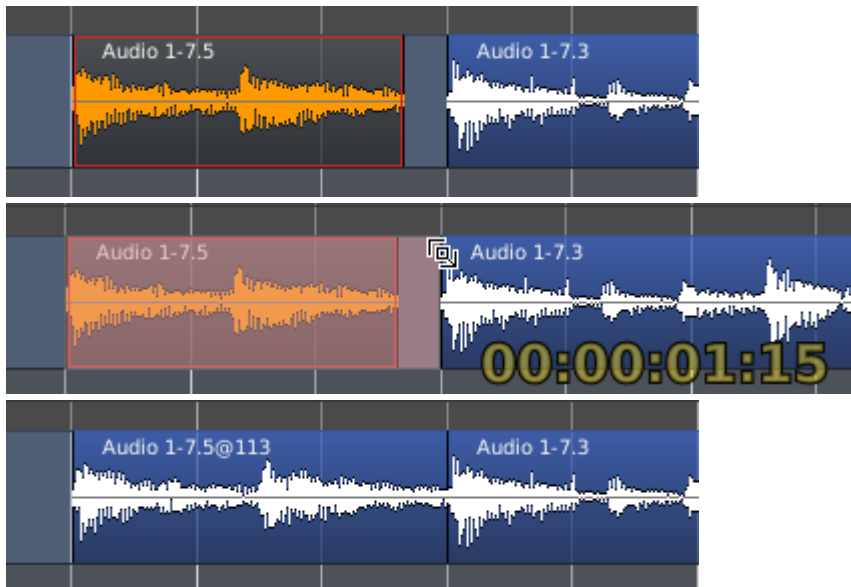
Fig. 49.3 - Using the Stretch Mode tool. Before stretching, while stretching, and after a stretch
