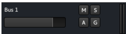
Fig. 29.5 - A bus header section
