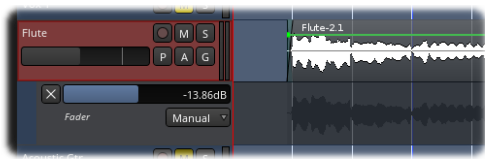
Fig. 71.3 - An example of a fader automation lane (below) with its associated track (above).
