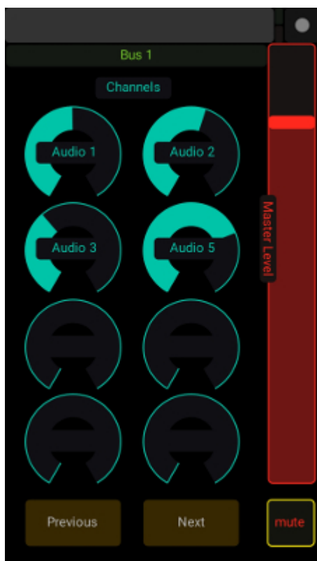
Fig. 65.8 - Personal Monitor controller using TouchOSC
