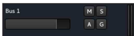
Fig. 29.5 - A bus header section
