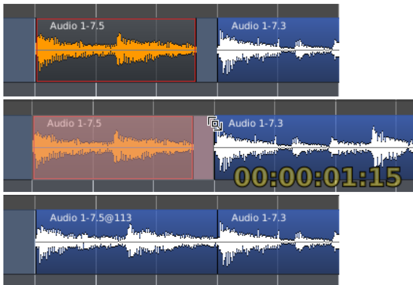
Fig. 47.3 - Using the Stretch Mode tool. Before stretching, while stretching, and after a stretch
